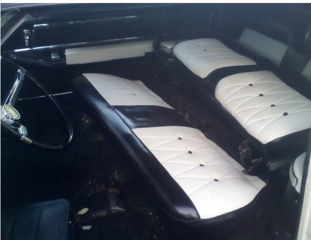
Bob's '64 Deville front bench seat dismantled ready for refurbishment
